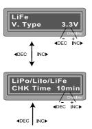
To change the default values, press the Start/ Enter key once. The value to be adjusted will blink indicating it can be edited. Use the Inc/Dec keys to adjust the value to the desired setting, then press the Start/Enter key once to save your changes for that value.
