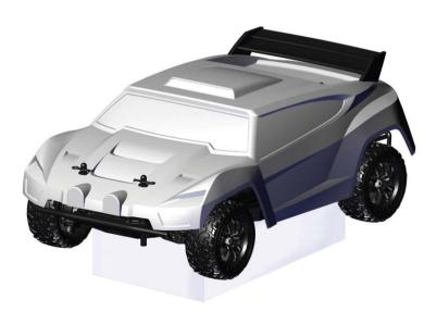
Perform a control test with the vehicle wheels off the ground. If the wheels rotate after the vehicle is powered ON, adjust the "TH. Trim" knob until they stop. To make the wheels move forward, pull the trigger. To reverse them, wait for the wheels to stop, then push the trigger. When moving forward, the wheels should maintain a straight line without any steering wheel input. If not, adjust the "ST. Trim" knob so the wheels maintain a straight line without having to turn the steering wheel.
