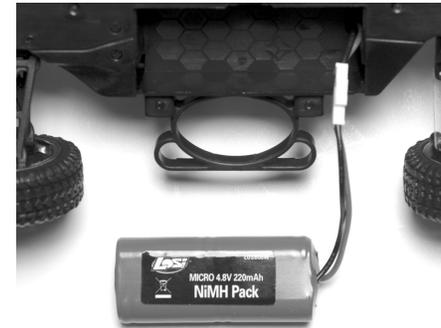
2. Plug the AC charger into the proper wall receptacle (110V - US version). Plug the battery pack into the charger and let it charge for 1 hour for the first time. Charge for 1 hour thereafter for a full charge. **Battery charged for over 1 hour may cause an overcharge.**
