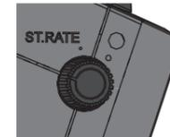
Turn the ST RATE knob clockwise to increase the sensitivity.
